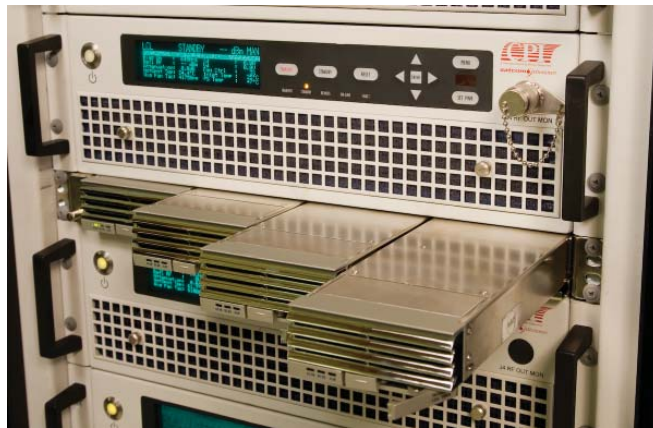
SSPA with optional redundant hot-swappable power supplies
